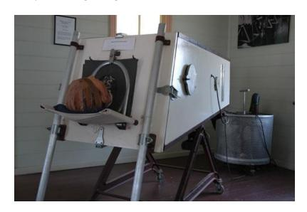
The image clearly shows both the 'tank' enclosing the patient and the bellows machinery at the bottom right of the photograph. The hose connecting the two is also visible. A flexible rubber seal surrounds the patient's neck.
